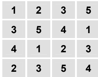
Figure 3.3: A 5-pin layout for a 4x4 array.
