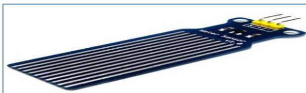
Figure 10. Physical representation of water sensor
