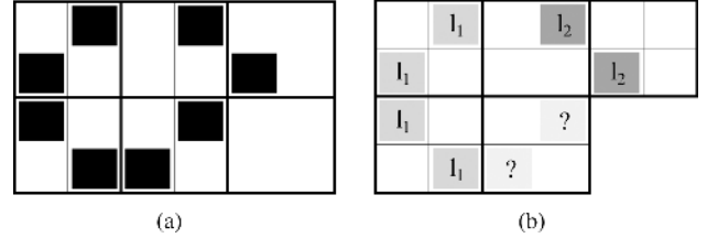
Fig. 8. Example of a complex merging situation: (a) the binary image and (b) the two sets of neighboring blocks with a common label.
