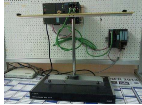
FIGURE 16: Ball and beam laboratory setup used in real time experiment.
