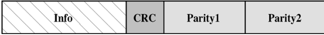
Fig. 3. Arrangement of data in a Turbo-coded row. Unlike in RCPC/CRC rows, data bits can be directly decoded if they are not corrupted.
