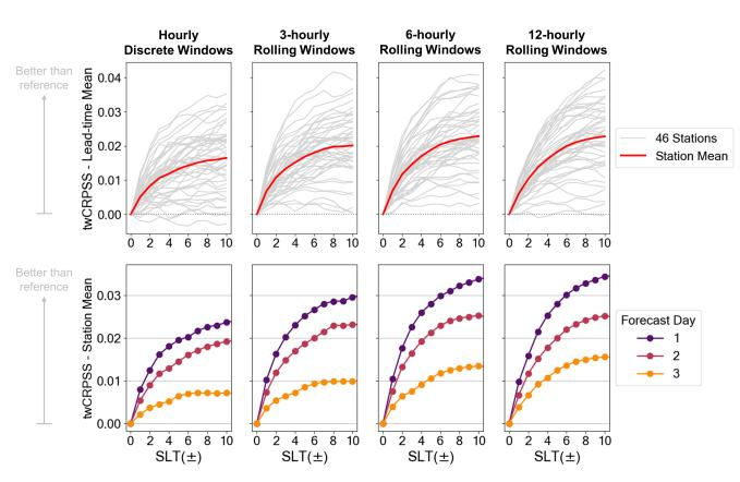
**Figure 7.** Lead-time aggregated (**top**) and station-aggregated (**bottom**) twCRPSS from the supplementallead-time (SLT) experiments. The reference for twCRPSS is the original approach with optimized predictors but without SLT. Positive twCRPSS indicate improvement compared to the reference.
