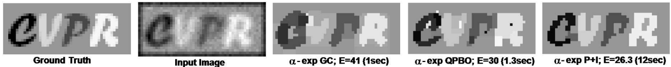
Figure 3. Image deconvolution. Given a blurry and noisy input image with 32 gray-levels, the task is to reconstruct the ground truth. The new P+I method within alpha-expansion improves results compared to graph cut and QPBO-based alpha expansion both in terms of energy and visually. Note, for all alpha expansion based methods the order is crucial. Energies of P+I differed between 26.3 and 27.9 and runtime between 12 and 31 sec, best result shown. Also, to improve runtime of P+I we initialized it with standard graph cut based alpha expansion. BP (E=103), TRW (E=112) and ICM (E=54) perform poorly. Simulated annealing achieved a similar result to P+I in 60 sec.
