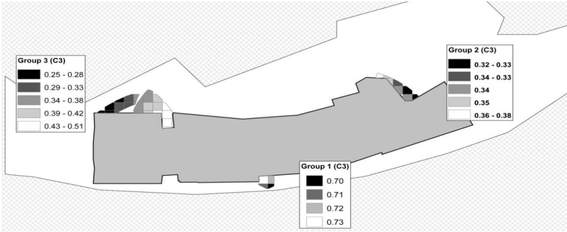
FIG. 6: Optimal locations of tower crane type 1 based on conflict index (C3)
