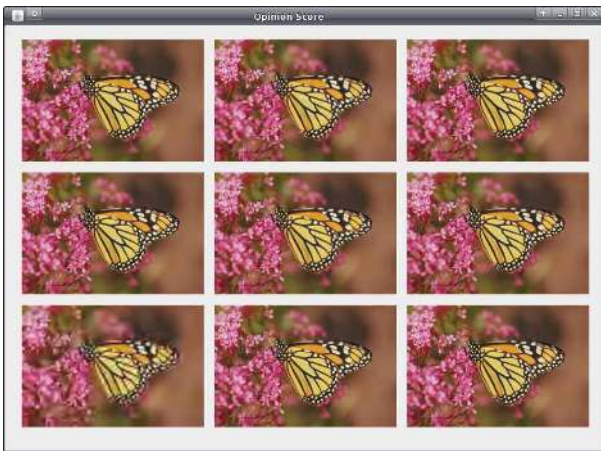
Fig. 4. Example of a single trial during the ordering test. The subject sees an image at the nine trial compression rates. The stimuli are randomly arranged on three lines. The subject was asked to order the quality of all images from the best to the worst quality.
