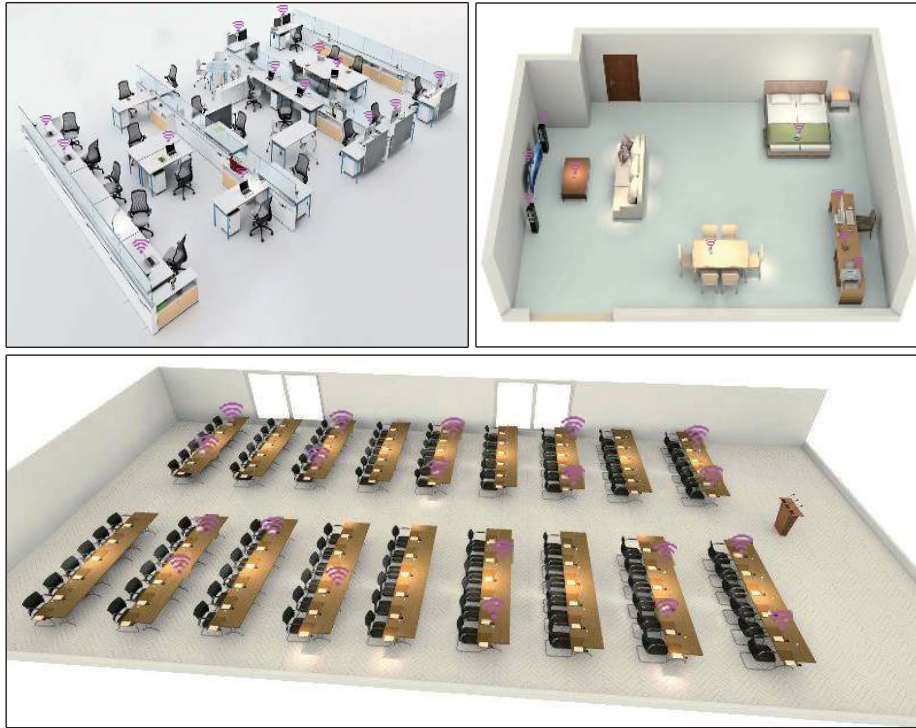
Figure 1.1: Dense wireless network deployment scenarios.
