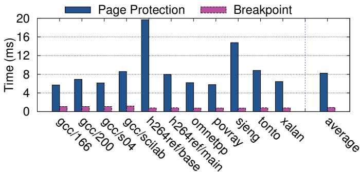
Figure 3.3. Overhead per sample for breakpoint and page-protection sampler. Page-protection has high overhead because of false-positives. Breakpoint based sampler is 10× faster than page-protection.
