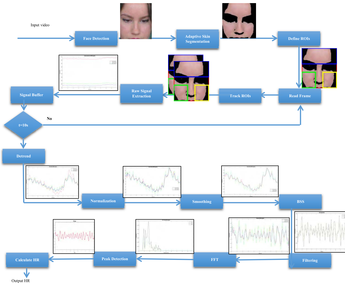
FIGURE 3. Flowchart of the proposed algorithm using adaptive ROIs.
