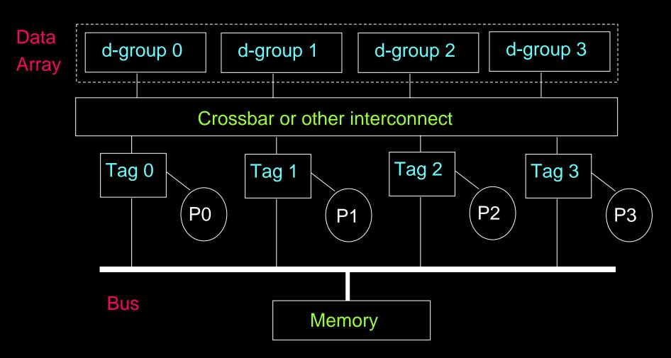
Tag arrays snoop on a bus to maintain coherence
