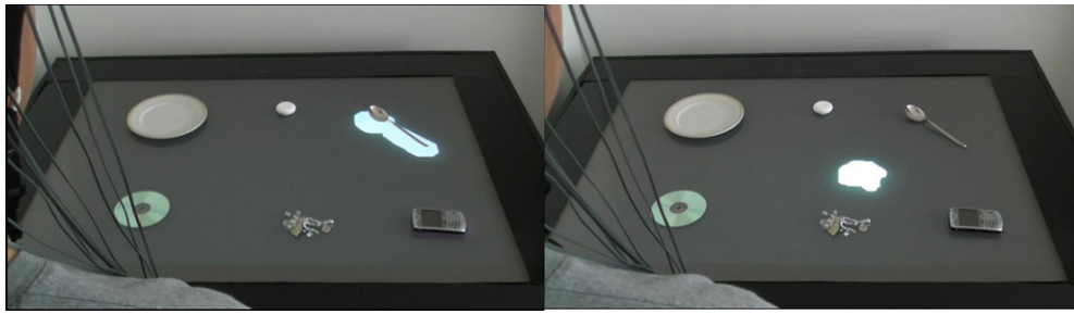
Figure 1. A participant using the P300-based BCI with real-world objects on a multi-touch surface. Left: the spoon is being flashed by surrounding the area underneath it with light; Right: a non-object flash. (This figure is in colour only in the electronic version)
