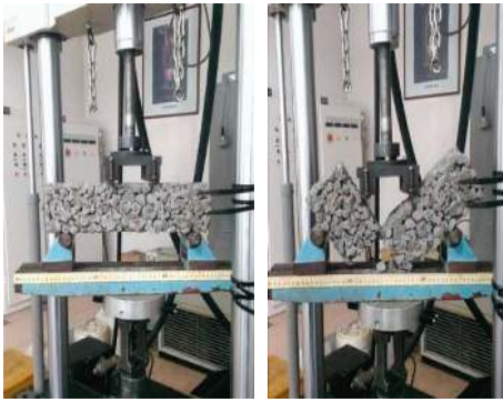
FIGURE 16: Flexural tensile strength tests.
