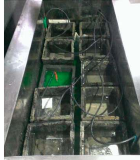
FIGURE 11: Frost resistance test.
