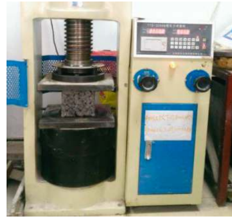
FIGURE 14: Compressive strength test.
