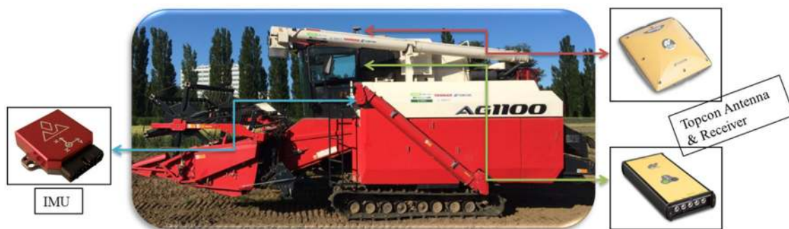
Fig. 2 Robot combine harvester with RTK-GPS position and IMU direction sensors
