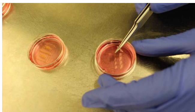
Movie S1. Manual transfer of muscle ring from injection mold to bio-bot skeleton. Muscle rings are lifted from the injection mold using sterile tweezers and transferred to another dish containing the bio-bot skeletons (chemically bonded to an underlying glass slide). The muscle ring is tethered around the bio-bot skeleton on day 1 after seeding.
