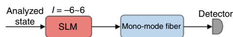
Fig. 7 The scheme of orbital angular momentum mode analysis. SLM spatial light modulator.
