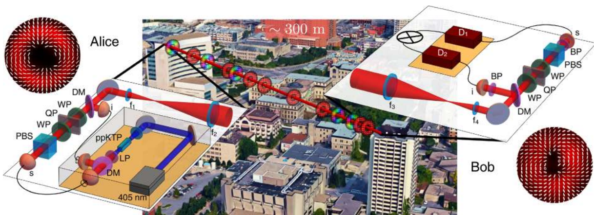
FIG. 45. The quantum communication link between two buildings over 300 m. ppKTP: periodically poled KTP crystal; LP: long-pass filter; WP: waveplate; BP: bandpass filter; DM: dichroic mirror. Reproduced with permission from Sit et al. , Optica 4, 1006 (2017). 201 Copyright 2017 Optical Society of America.
