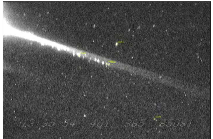
Figure 6. Identification of reference stars and debris fragments using TrackEye software.
