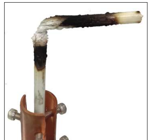
Figure 2. Sample of axially oriented GFRP inserted in argon plasma for 80 seconds (considered demised).
