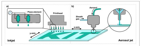
**Figure 6.** Schematic description of the functionality of digital printing techniques. (a) Inkjet printed structures are formed a pattern from adjacent single droplets that are being ejected from the nozzle head on demand. (b) Aerosol jet printing a high-resolution spray coating, Where an atomized ink is focused by a sheath gas stream. For both techniques either the printhead or substrate movement allows for 2D structuring.
