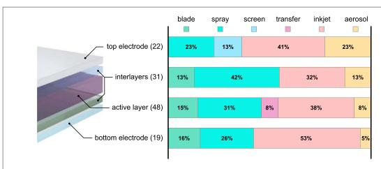
**Figure 3.** Usage of the different printing and coating techniques for the fabrication of the different OPD layers. The total number of reports per layer is included in parentheses.
