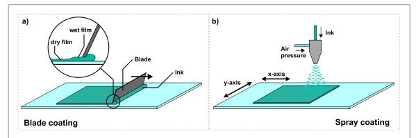
**Figure 4.** Coating techniques that have been employed for OPD layer fabrication. (a) Blade coating makes use of a blade or bar, which drags an ink continuously across a substrate, leaving a wet film that dries to form the desired layer. (b) Spray coating involves the generation of a tiny droplets which are deposited through a nozzle onto the substrate. 2D-deposition is possible through *x*–*y*-movement of the spraying apparatus or the substrate.
