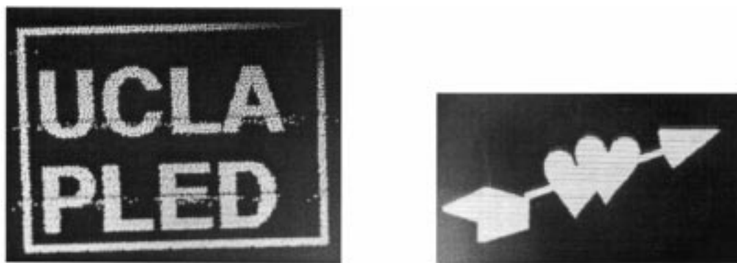
Figure 4 The polymer light emitting logo patterned by the IJP technology; (a) a UCLA logo, and (b) a valentine hearts logo.
