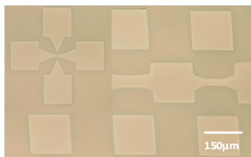
Figure 4. Optical micrograph of the conducting polymer PEDOT pattern on PET flexible substrate by using a roll-to-roll printing machine. The inset shows the transferred PEDOT pattern with 5 \mu\text{m} channel gap.
