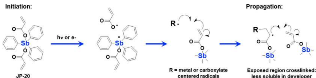
Fig. 12 Proposed mechanism of antimony organometallic carboxylate resist system. We propose that good sensitivity is achieved through one photochemical homolysis event leading to a cascade of subsequent solubility changing polymerization reactions.
