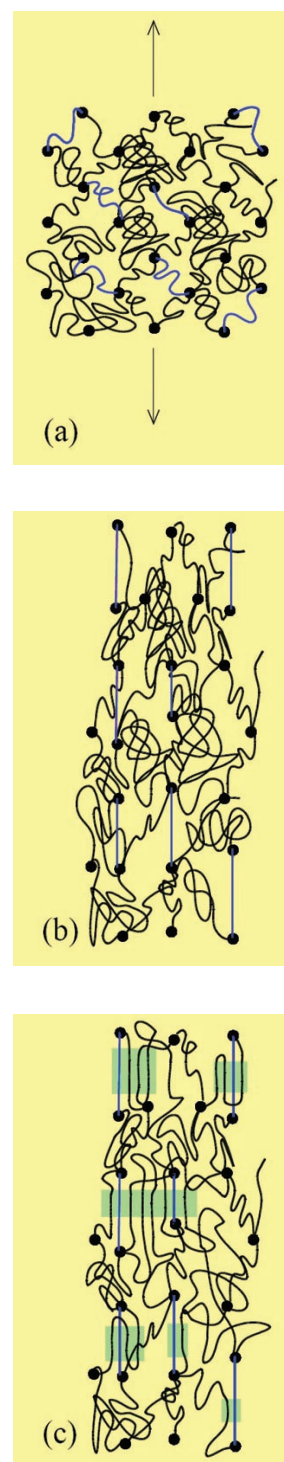
Figure 1. A model of the strain-induced crystallization in vulcanized NR. Relatively short chains are drawn as blue lines. Filled circles represent crosslinks. (a) Before deformation. (b) After deformation: Short chains are fully stretched. (c) Crystallites are grown from the stretched chains (green parts).
