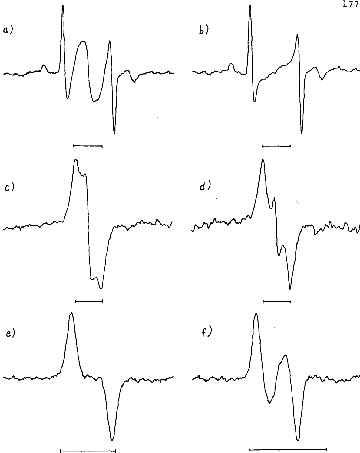
Fig. 42 Derivatives of the absorption signal with [(a), (c), and (e)] and without [(b), (d), and (f)] the ^1\text{H} background signal. A=13 dB and \bar{\beta}=0^\circ . The horizontal bars are 2 mT. The total measuring time is t_m . (a) and (b): .318 K, t_m=1.2 h, c=.95 . (c) and (d): .664 K, t_m=2.4 h, c=.91 . (e) and (f): .860 K, t_m=1.2 h, c=.89 .
