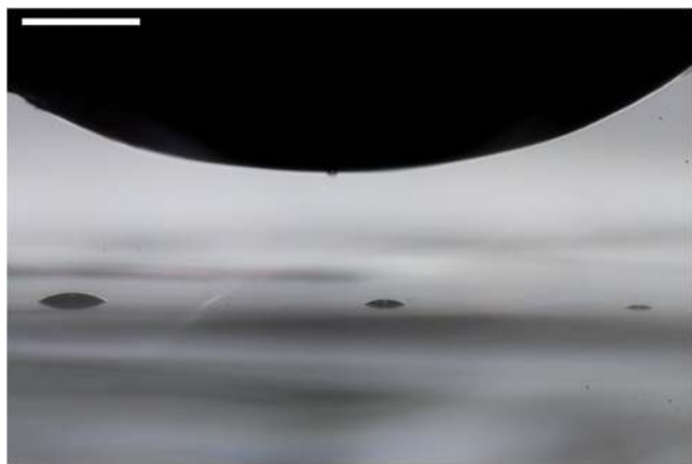
Fig. 4 Deposition of nematic liquid crystal droplets on the mica substrate using a polytetrafluoroethylene rod. The scale bar in the upper left corner denotes 500 \mu\text{m} .
