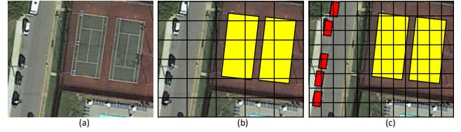
Fig. 3: Multi-scale on-off strategy on a sample image; a) ground-truth, b) objects which are smaller than the cell become 'off', c) objects (shown in red) become 'on' in a smaller cell.
