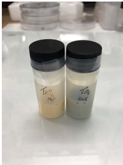
Figure S4. \text{TiO}_2 and \text{TiO}_2 -CNT sol gel solutions used for the mp- \text{TiO}_2 layer in PSCs
