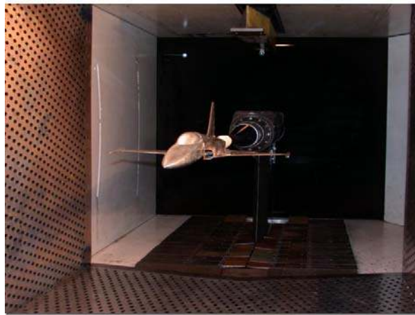
Figure 18. High-speed model installed in AEDC's 4' supersonic wind tunnel.
