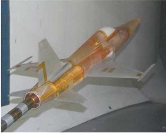
Figure 17. Low-speed model undergoing tests in NGC's 7' x 10' wind tunnel.
