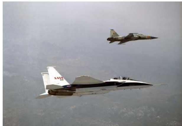
Figure 13. Inlet spillage shock measurement of baseline F-5E with NASA F-15B probe aircraft.
