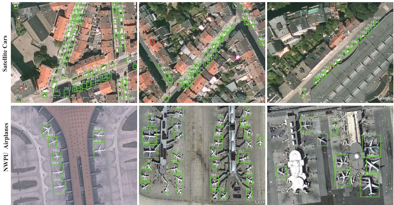
Fig. 8. Some visual detection results (false detection in red box, TP in green box, and missing detection in blue box) by using the proposed method on the two different data sets.
