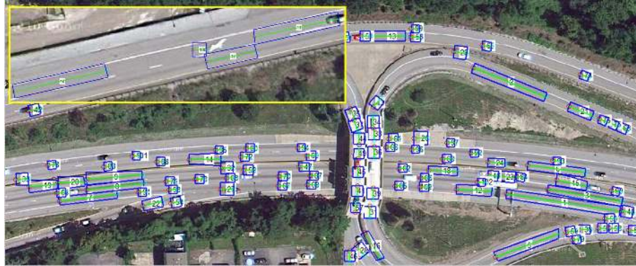
(b) The road-lane hypothesis generation process produces 99 hypotheses about the 10 true road-lanes.
