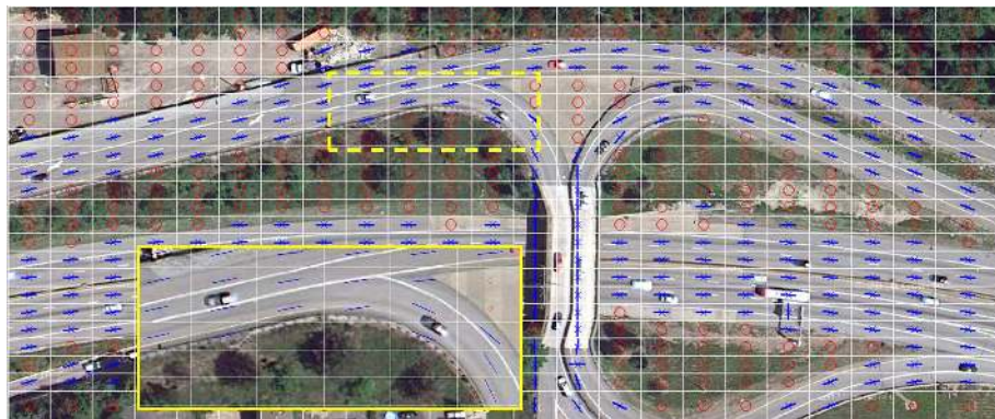
(b) Results of driving direction estimation. The blue lines indicate the estimated driving direction of a grid cell and the non-drivable regions are depicted by red circles.
