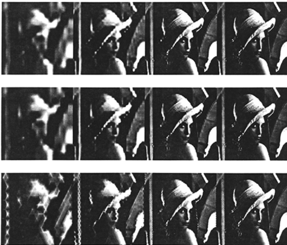
Figure 12: Progressive transmission with three types of pyramid. Top row: 9-tap QMF pyramid. Bit rates for the 9-tap sequence are: 0.03, 0.09, 0.24, 0.49 bit/pixel. Rates for the other sequences are essentially the same. The final image, at 0.65 bit/pixel is not shown (see fig. 11).
