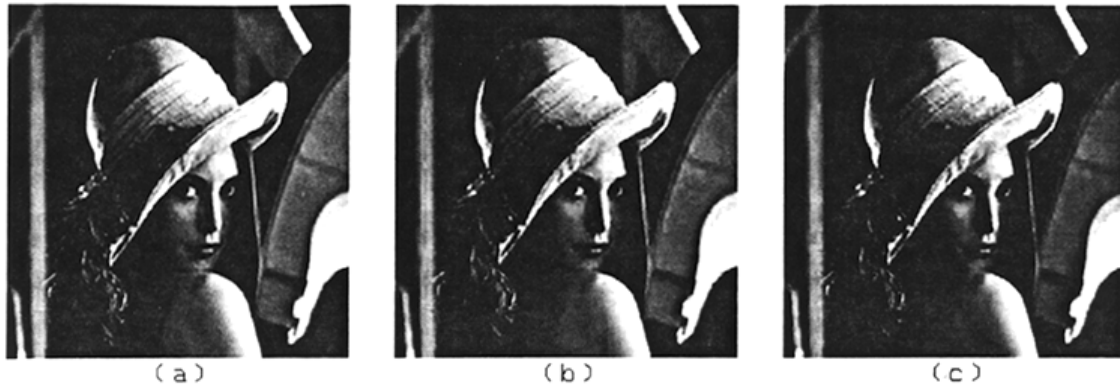
Figure 11: Data compression of the 256x256 Lena image. (a) Original. (b) 9-tap pyramid, 0.85 bit/pixel. (c) 3-tap pyramid, 0.65 bit/pixel.
