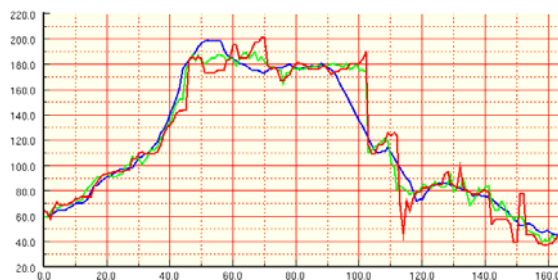
Fig. 8: Comparison of disparity values for classical method (blue), semiglobal matching (red) and fused method (green)
