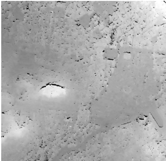
Fig. 3: DSM generated with the fused algorithm (digital line warping and semiglobal matching)
