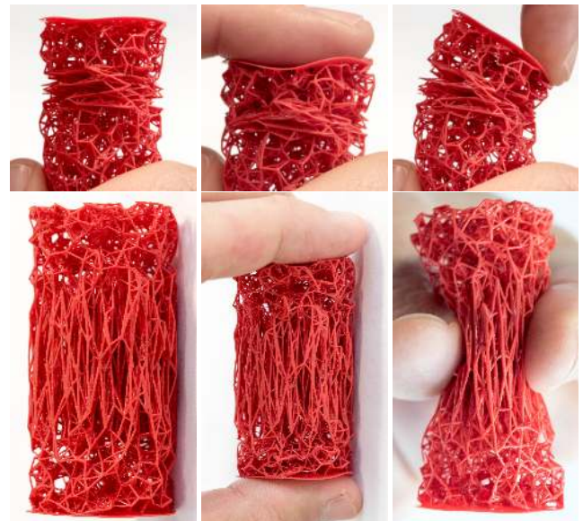
Fig. 15. 3D printed cylinders with orthotropic material. Top: The center segment is made more rigid horizontally and flexible vertically. Bottom: The extremities are isotropic, the center is rigid along the main axis but flexible radially.
