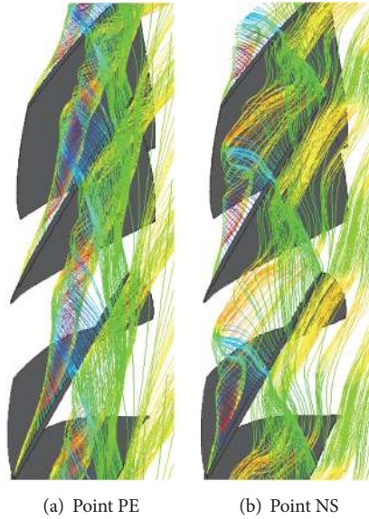
FIGURE 3: Streaklines that depict the TLF structures ([12]). Figure reproduced from LIN et al. (2010).
