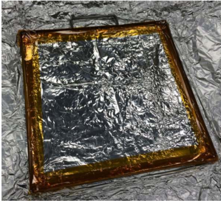
Fig. 5. Amino acid contamination monitoring plate adapted from a standard 1 × 1 ft. ASTM E1235–12 NVR plate for the 4-m Atlas V fairing
