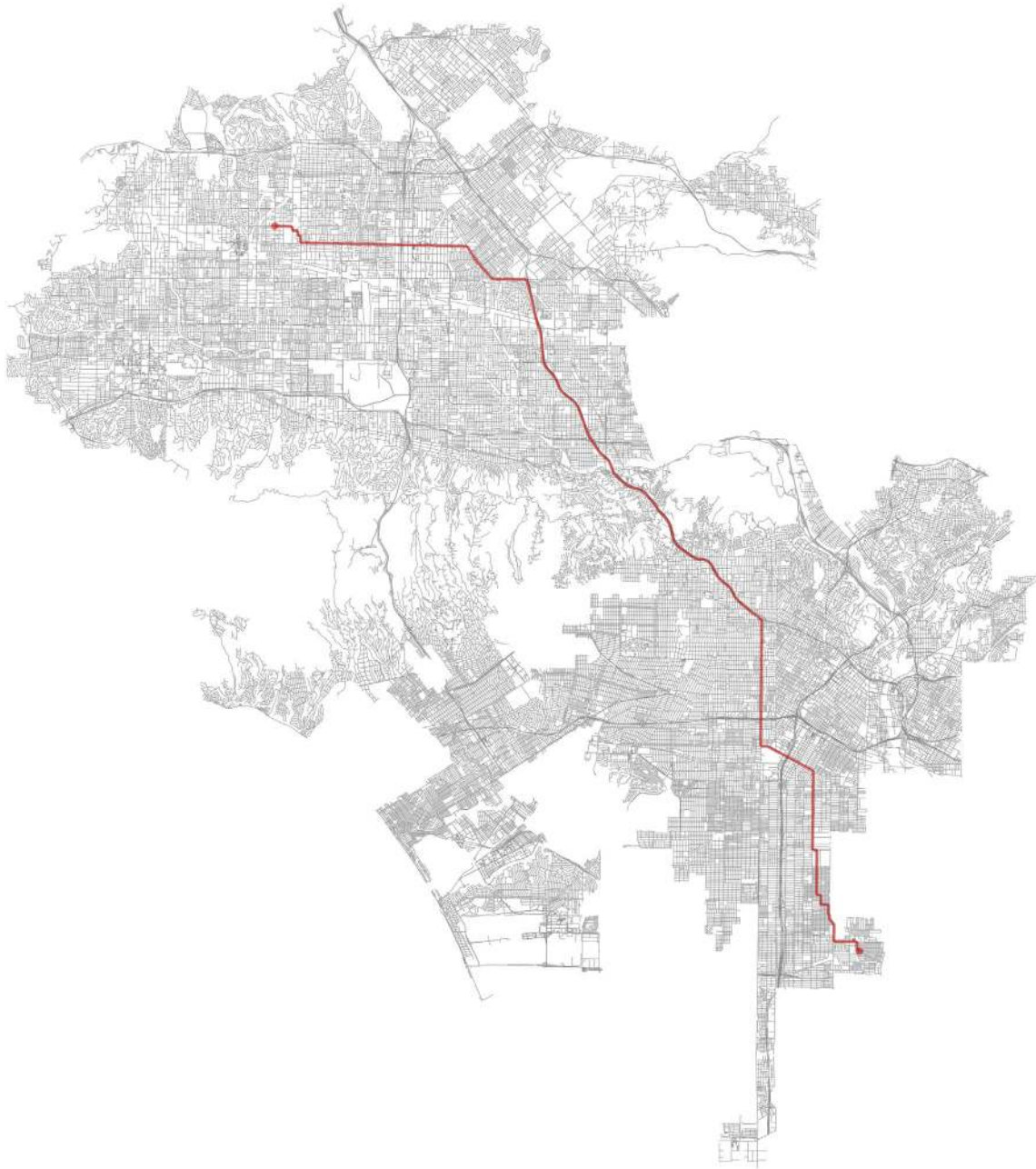
Fig. 7. OSMnx calculates the shortest network path (weighted by edge length) between two points in Los Angeles, accounting for one-way routes, and plots it.
