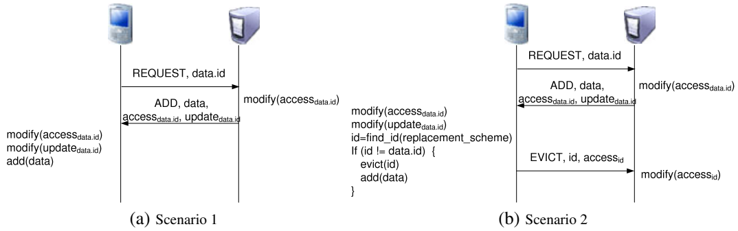
Figure 4. Steps for Update-based Call-Back access scheme in different scenarios at a cache miss: (a) Scenario 1 and (b) Scenario 2.
