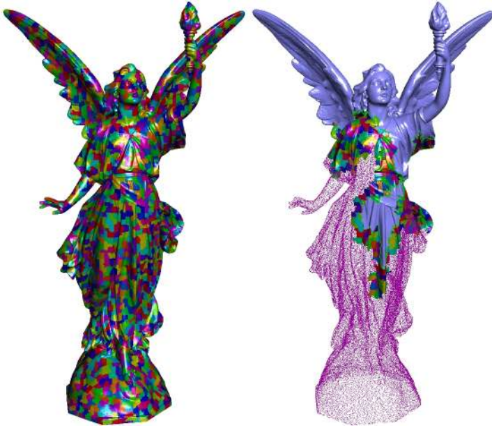
Figure 3: Visualization of the clustering and its usage during compression on the Lucy statue with S_{\text{incore}} = 64\text{MB} and c_{\text{cache}} = 128 . Already encoded regions are rendered with points while the rest is rendered with triangles. Cached clusters are colored.
