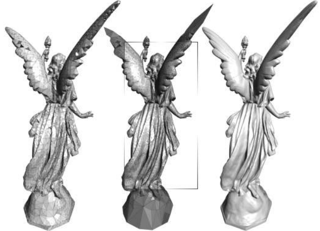
Figure 1: Various view-dependent meshes produced by our system. The mesh in the middle has been coarsened aggressively outside the view frustum (here shown as a rectangle).
