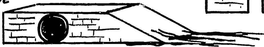
RAMP AND TUNNEL OF CEMENT BLOCKS, CULVERTS
