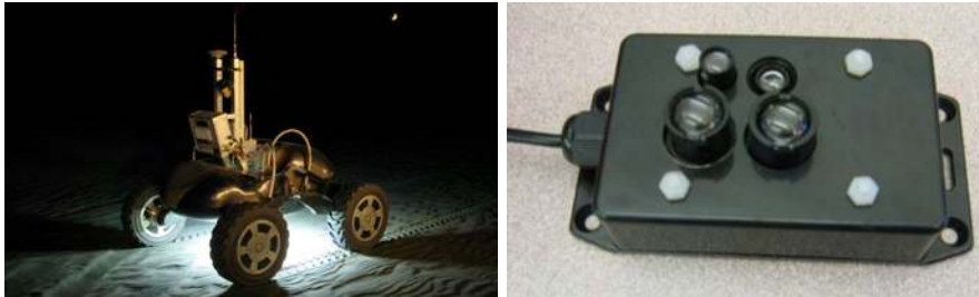
Fig. 1 The Scarab lunar rover. The glow beneath Fig. 2 The optical sensor used on Scarab, in a custom ruggedized enclosure.
