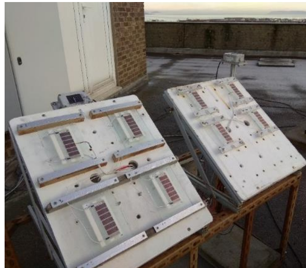
95 96 Figure 2 - Outdoor monitoring setup used to perform the tests in (a) Belo Horizonte, Brazil, at an angle of 20°, facing 97 North, and (b) Bangor, Wales, with an inclination of 35°, facing South. The already existing installations and 98 measuring systems were used.
