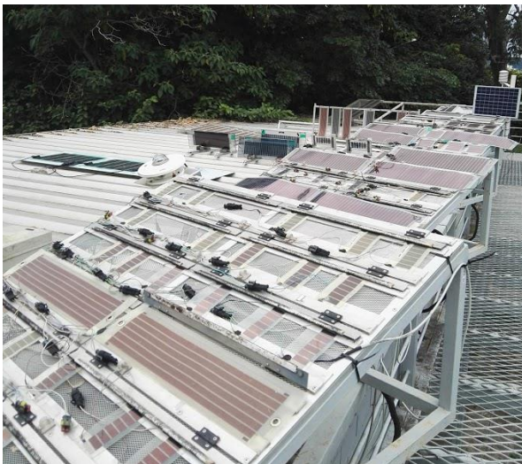
95 96 Figure 2 - Outdoor monitoring setup used to perform the tests in (a) Belo Horizonte, Brazil, at an angle of 20°, facing 97 North, and (b) Bangor, Wales, with an inclination of 35°, facing South. The already existing installations and 98 measuring systems were used.
