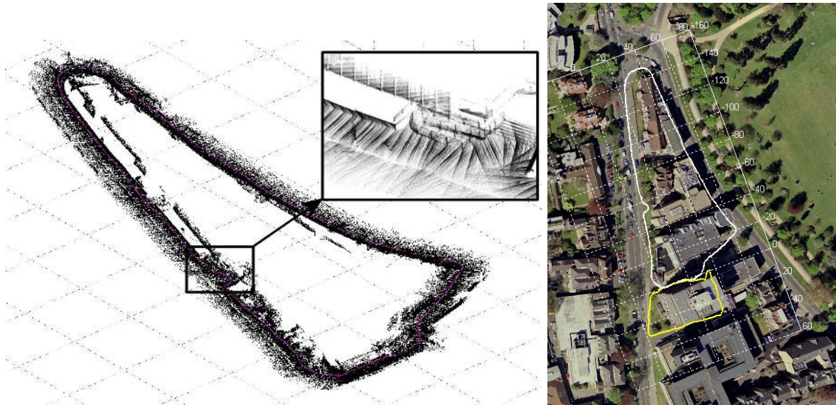
Fig. 9. The resulting estimated map and vehicle trajectory. The inset shows some local detail within the map which contains just over four million range points and the trajectory is decomposed into just over four hundred 6DOF poses. The intersection between the independently executed loops was found in the same way that the loop closures themselves were found - sequential appearance based similarity as described in Section III.
