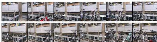
Fig. 8. Automatically detecting overlapping maps by comparing image sequences observed by different vehicles. The top row is the sequence observed from the vehicle executing the white (upper) loop in Figure 9 while the bottom row is the matching sequence captured by the vehicle that executed the yellow (lower) loop. This matching corresponds to the off diagonal band in Figure 7.
