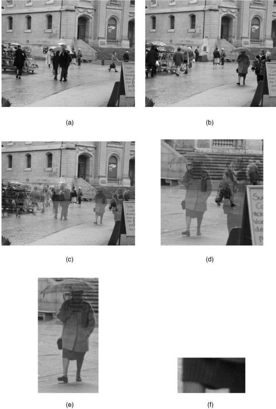
Fig. 5. (a) and (b) Original pictures used to perform outlier detection tests. (c), (d), (e), and (f) Ghost pictures used to perform the outlier tests. The images are superimposed using transparency; hence, the outliers appear as a ghost image. (c) The whole image, (d) region of picture (c), (e) region of picture (d), and (f) region of picture (e). The subimages are chosen such that the part of the image covered by the outliers is increasing.
