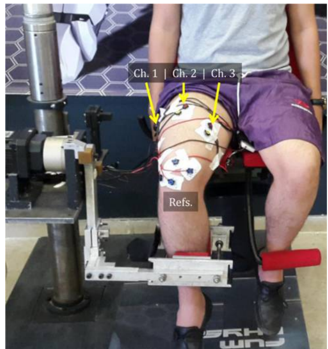
Figure 14 The subject on FUM-Physio and the location of sEMG electrodes
