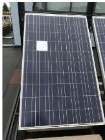
Fig. 6. Opaque paper object covering one solar cell
