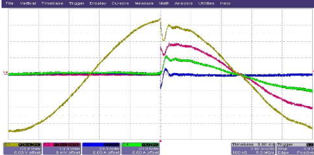
Fig. 13. Output voltage (yellow), load current (red, x2), inductor current (green), capacitor current (blue) transients (Scales: 50V/div, 20A/div, 2ms/div).
